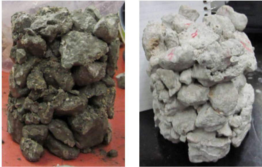
Figure 110. MI I-96 CTB wet-dry durability sample #2 before (left) and after (right) testing
