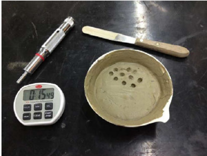
Figure 278. Set time test on Ames, IA Municipal Power Plant fly ash
