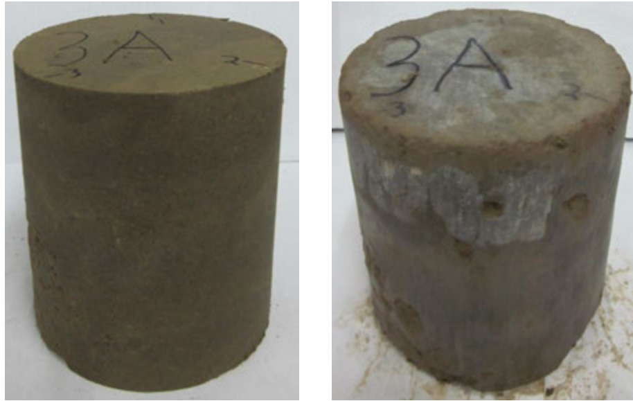
Figure 127. Cement-treated loess freeze-thaw durability sample #3 before (left) and after (right) testing
