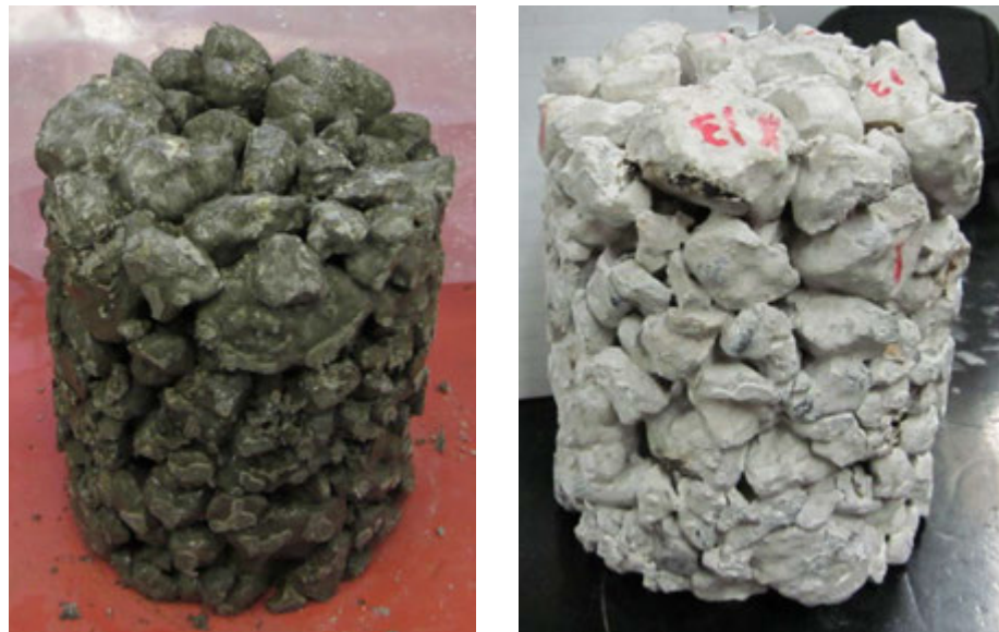
Figure 109. MI I-96 CTB wet-dry durability sample #1 before (left) and after (right) testing
