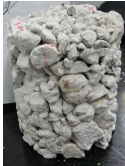
Figure 114. MI I-96 CTB freeze-thaw durability sample #4 before (left) and after (right) testing
