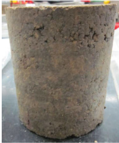
Figure 103. IA I-29 lean clay subgrade wet-dry durability sample #1 before testing
