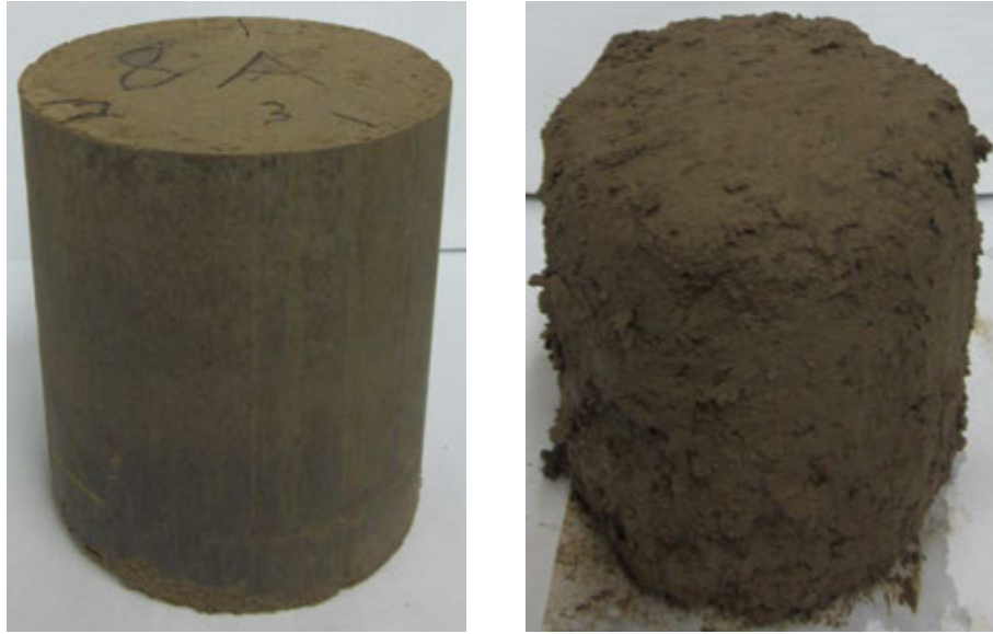
Figure 134. Fly ash-treated loess freeze-thaw durability sample #8 before (left) and after 8 th cycle (right) testing
