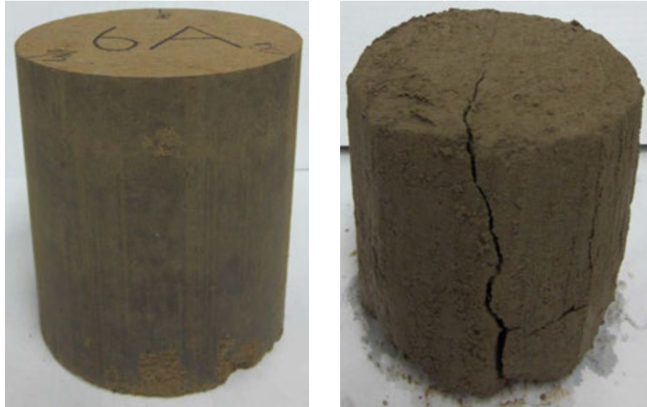
Figure 132. Fly ash-treated loess freeze-thaw durability sample #6 before (left) and after 7 th cycle (right)
