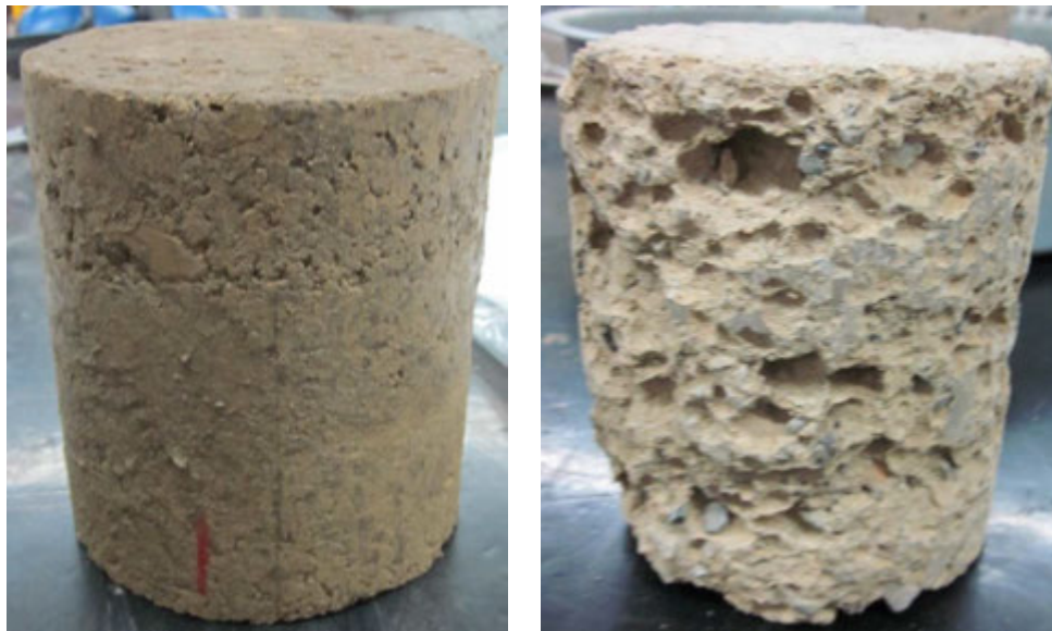
Figure 119. PA US-22 sandy lean clay subgrade wet-dry durability sample #1 before (left) and after (right) testing
