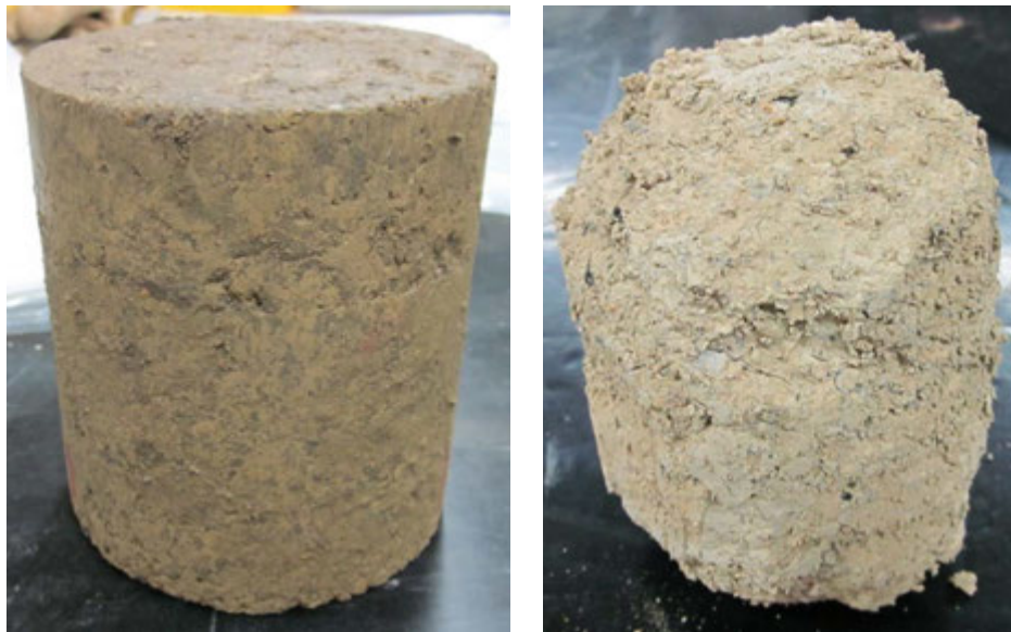
Figure 122. PA US-22 sandy lean clay subgrade freeze-thaw durability sample #2 before (left) and after (right) testing
