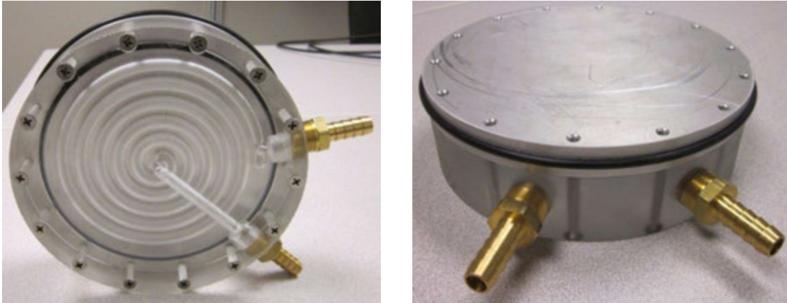
Figure 42. Acrylic side (left) and aluminum side (right) of temperature control end plate used to freeze and thaw samples
