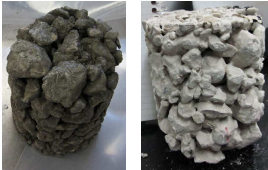
Figure 116. MI I-96 CTB freeze-thaw durability sample #6 before (left) and after (right) testing
