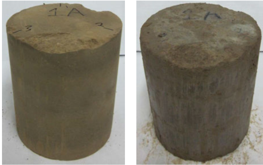
Figure 125. Cement-treated loess freeze-thaw durability sample #1 before (left) and after (right) testing
