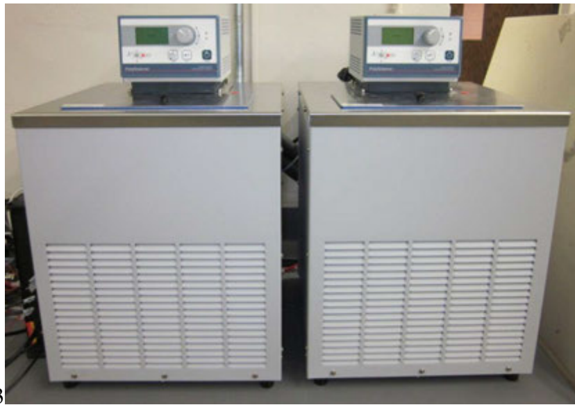
Figure 44. Temperature control baths used to freeze and thaw samples
