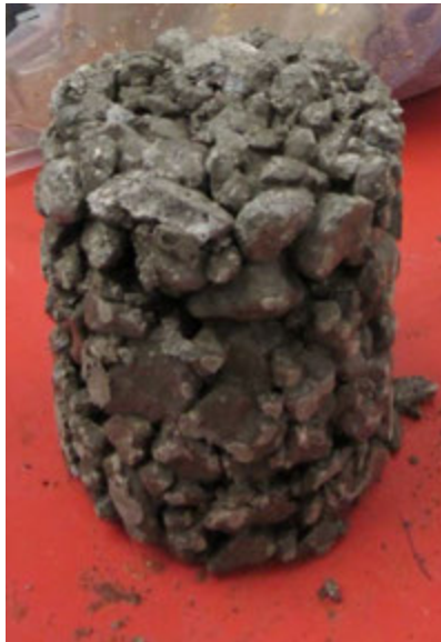
Figure 114. MI I-96 CTB freeze-thaw durability sample #4 before (left) and after (right) testing
