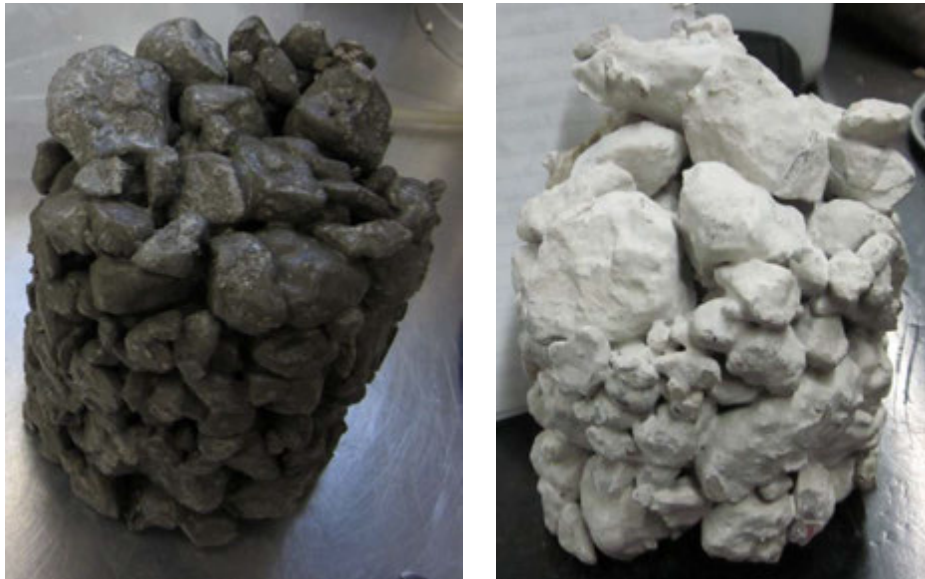
Figure 111. MI I-96 CTB wet-dry durability sample #3 before (left) and after (right) testing
