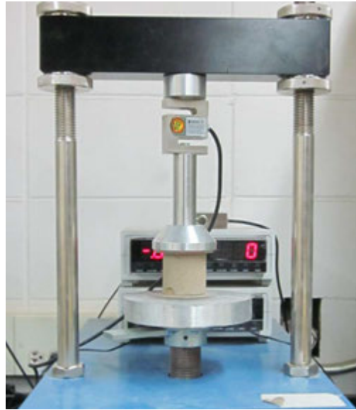
Figure 32. 2-in. x 2-in. unconfined compression test
