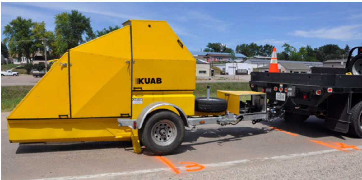
Figure 53. Falling weight deflectometer (FWD) test
