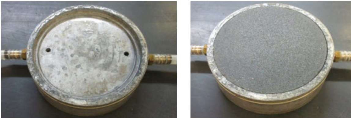
Figure 43. Sample base plate without porous stone (left) and with porous stone (right)
