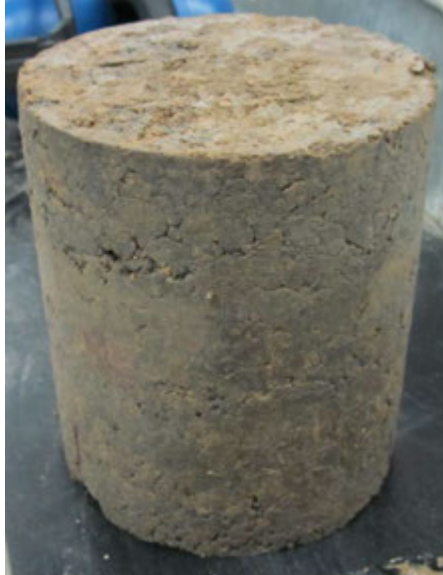
Figure 106. IA I-29 lean clay subgrade freeze-thaw durability sample #2 before testing
