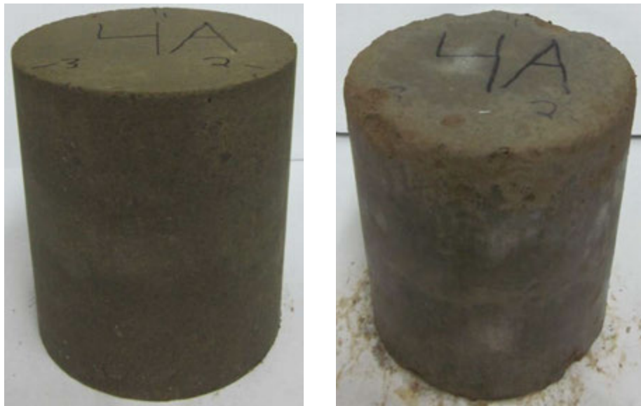
Figure 128. Cement-treated loess freeze-thaw durability sample #4 before (left) and after (right) testing
