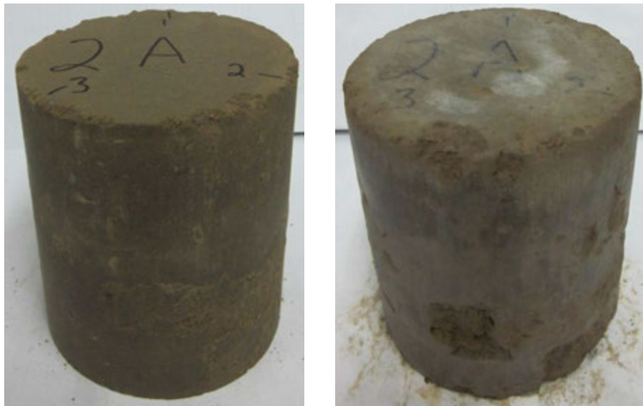
Figure 126. Cement-treated loess freeze-thaw durability sample #2 before (left) and after (right) testing
