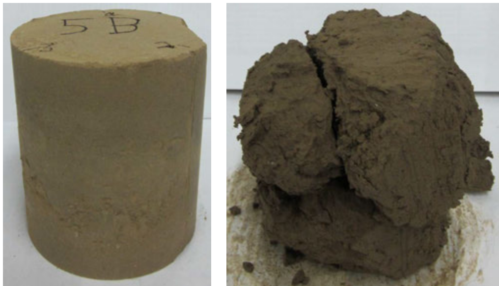
Figure 131. Fly ash-treated loess freeze-thaw durability sample #5 before (left) and after 3 rd cycle (right)
